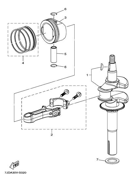
FIG. 2 CRANKSHAFT & PISTON
